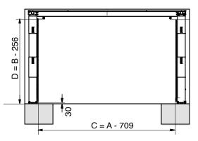
A = aperture width; B = aperture height; C = free opening width; D = free opening height
