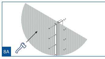
Overlap mesh on intermediate post. Clamp into place using flat bar and insert bolts from attack side.
