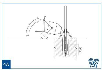
Fill foundations with concrete up to 750 mm depth.
