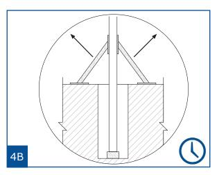
Allow concrete to cure. Remove wooden struts.
