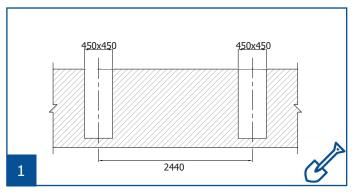
Clear and level the site appropriately before beginning installation. Calculate foundation dimension - see Appendix. Dig holes accordingly.
