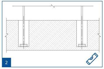
Insert posts, using a spirit level to keep them perpendicular. If necessary, place wooden blocks at base of posts to keep them flat and level with one another.
