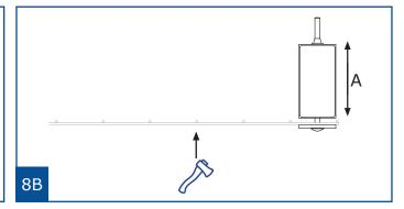
Assemble bolts as shown. Bolts should be 30 mm longer than dimension A. Refer to Appendix to determine this.
