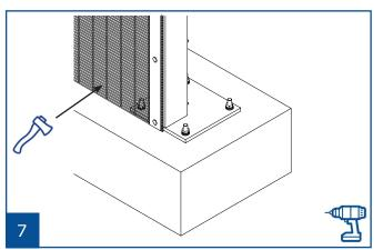
For installations with baseplates, see details on the site drawings. A standard baseplated system is shown above (with 15 mm diameter fixing holes).
