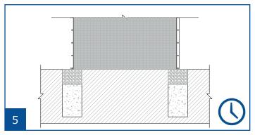
Affix panels to posts as shown in section 4.5. Fill remainder of foundations.
