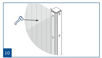
Fix the mesh to the exterior of the posts.
