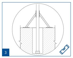
Attach wooden struts to hold the posts in place.
